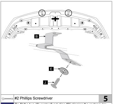
Re-fit the two (2) center fixed clips "B" aligning the rectangular holes in the clips with the previously installed screw plugs "D". Insert the two (2) self tapping screws "J" through the two (2) washers "E" into the two (2) screw plugs "D", as shown. Make sure that the clips rest on the abrasive resistant tapes.
