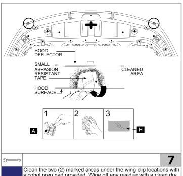
Clean the two (2) marked areas under the wing clip locations with alcohol prep pad provided. Wipe off any residue with a clean dry cloth. Align the large abrasive resistant tape "H" so that center of tape is aligned with wing clip screw hole in deflector. Apply the large abrasive resistant tape "H" so that approximately one third of the strip is adhered to the top side and two thirds is adhered to the underside of the hood.
